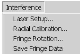
The Interference menu provides access to XL-I interference optical system controls.
