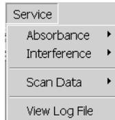
The Service menu provides read-only access to factory-set hardware and calibration settings. If troubleshooting is necessary, you can view the service windows and provide the information to a Beckman Coulter representative. To change service settings, a password is required.
